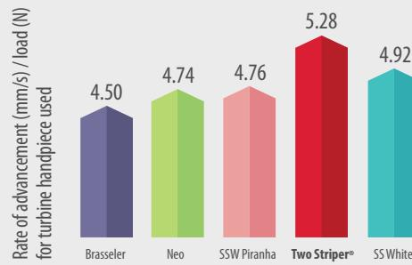
"Because advancement rate and load are interrelated (in general, the application of higher loads should lead to more rapid advancement), combining the two parameters provides an overall indicator for the ease of advancement of the rotary cutting instrument inside the substrate. Indeed, a significant difference was found between the Two Striper and the other rotary cutting instrument groups."
